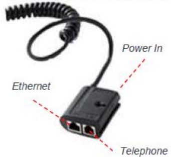
Connecting the Desk/5000 magic box to power and communication cables
